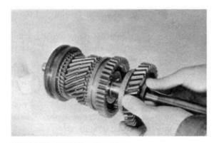
Fig. 2-181 Installing First Gear
