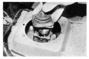
Fig. 2-145 Removing Shift Lever
