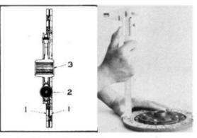
Fig. 1-21 Clutch Disc Inspection
