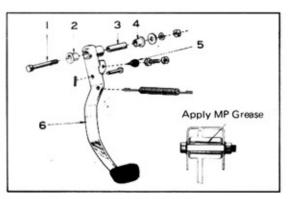
Fig. 1-7 Installing Clutch Pedal
