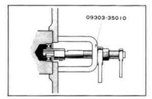
Fig. 1-26 Removing Bearing
