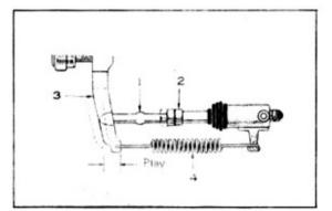
Fig. 1-9 Removing Release Cylinder
