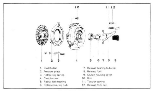
Fig. 1-17 Clutch Assembly
