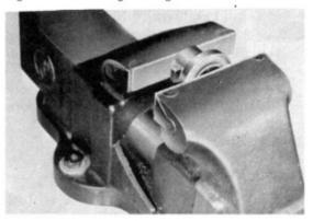
Fig. 1-25 Installing Bearing
