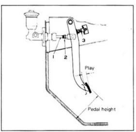
Fig. 1-2 Pedal Adjustment
