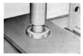
Fig. 1-24 Removing Bearing
