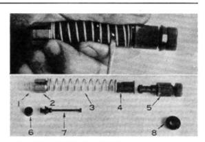
Fig. 1-14 Disassembling Piston
