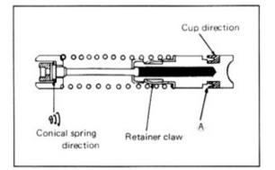
Fig. 1-16 Assembling Piston
