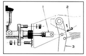
Fig. 1-12 Removing Master Cylinder
