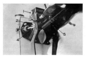
Fig. 1-6 Removing Clutch Pedal
