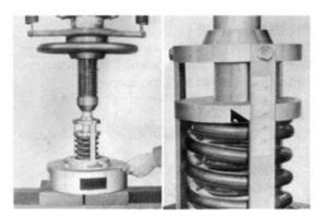
Fig. 1-19 Measurement of Installation Load
