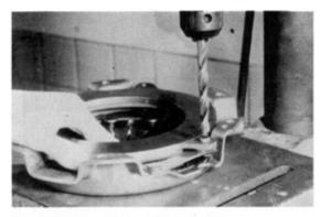
Fig. 1-20 Clutch Cover Disassembly
