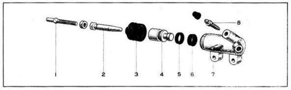
Fig. 1-8 Clutch Release Cylinder
