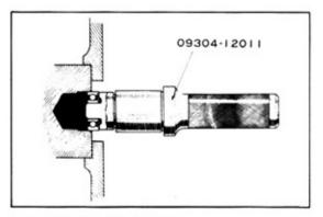
Fig. 1-27 Installing Bearing
