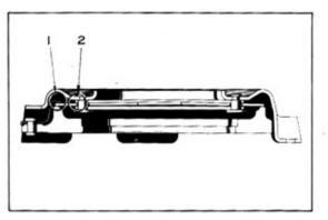
Fig. 1-28 Applying MP Grease
