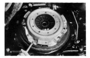
Fig. 1-31 Clutch Assembly
