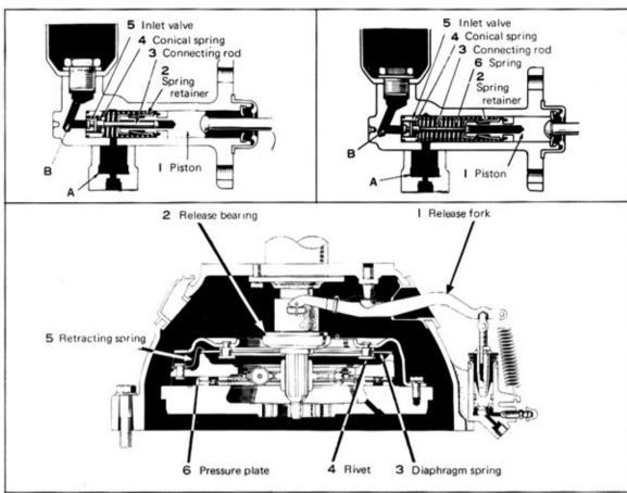
Fig. 1-1 Clutch System
