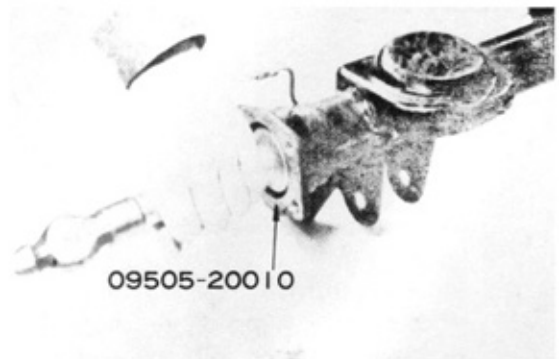
Fig. 4-47 Installing Oil Seal
