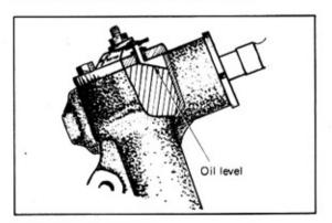
Fig. 7-34 Gear Oil Level
