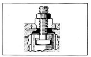
Fig. 7-22 Thrust Washer
