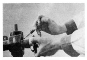
Fig. 7-30 Sector Shaft Reassembly
