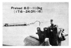
Fig. 7-31 Measuring Preload
