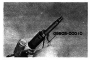
Fig. 7-9 Bearing Removal
