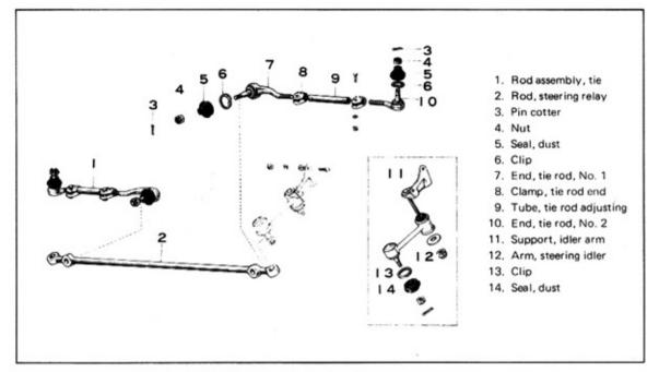
Fig. 7-35 Steering Linkage Component Parts
