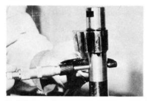
Fig. 7-21 Sector Shaft Inspection
