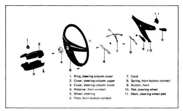
Fig. 7-3 Steering Wheel Component Parts
