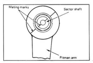
Fig. 7-33 Pitman Arm Alignment Marks
