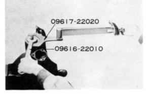
Fig. 7-29 Tightening Lock Nut
