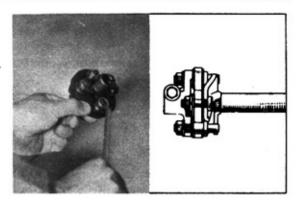
Fig. 7-10 Coupling Reassembly
