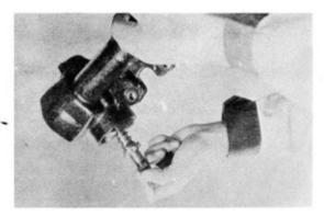
Take out the steering worm assembly together with bearing from out of the gear housing. Note: Do not disassemble the ball nut from the steering worm assembly. If defective, replace the entire assembly.
