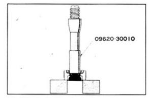
Fig. 7-26 Bearing Cup Removal
