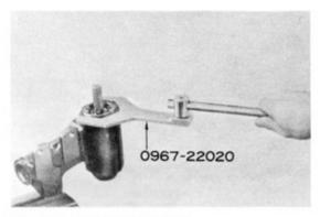
Fig, 7-17 Removing Lock Nut
