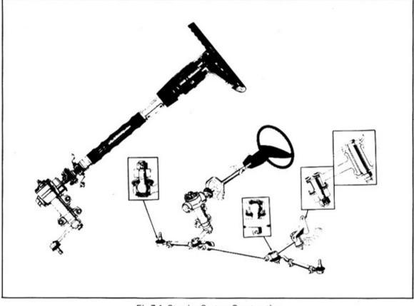
Fig 7-1 Steering System Construction
