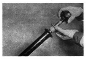
Fig. 7-11 Main Shaft Reassembly
