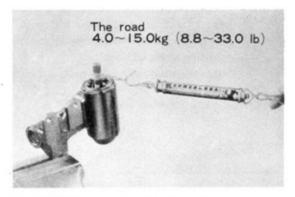
Fig. 7-28 Measuring Bearing Preload
