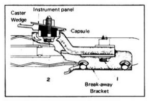
Fig. 7-12 Break-away Bracket Installation
