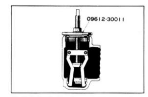
Fig. 7-25 Bearing Cup Removal
